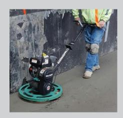
Allows finishing within 7/16" of any obstruction
